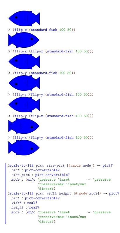
Scales *pict* so that it fits within the bounding box of *size-pict* (if two arguments are supplied) or into a box of size *width* by *height* (if three arguments are supplied).
