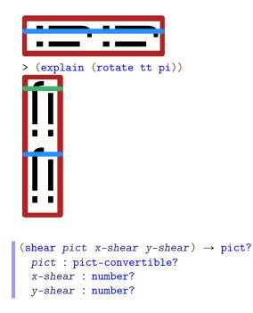
Shear's the *pict* by a factor of x-shear along the x-axis and by a factor of y-shear along the y-axis. The bounding box is inflated to contain the result. The result's ascent and descent are the same as *pict*'s.
